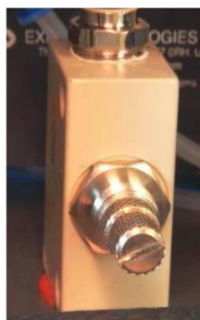
Figure 7 Leakage Compensation Valve (LCV)
